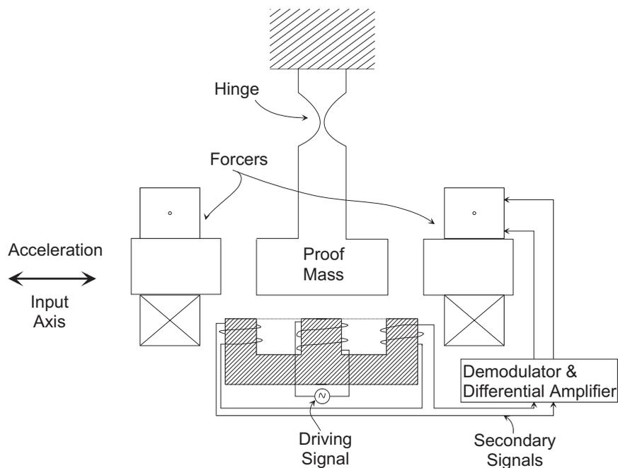
Figure 2.1: Generic pendulous accelerometer
