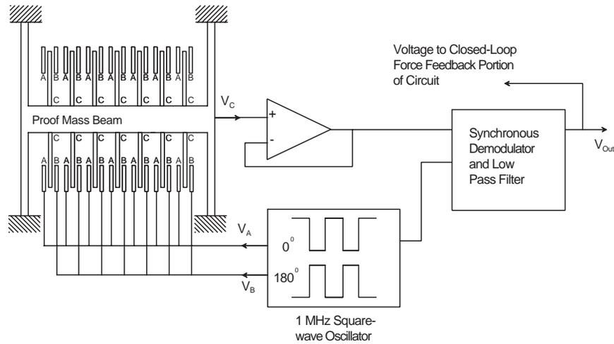
Figure 3.3: Schematic Illustration of ADXL05.
