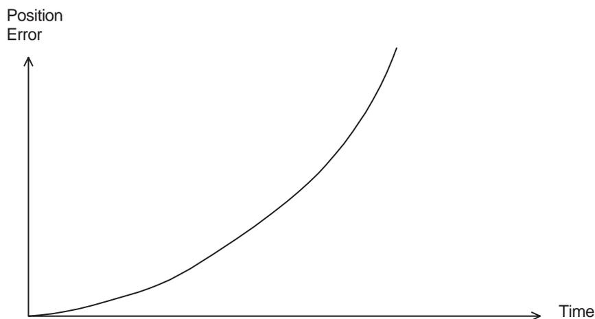
Figure 1.3: Characteristic positional error of inertial estimators.
