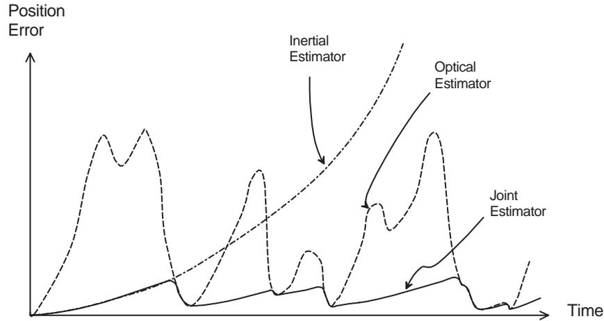
Figure 4.2: View of positional errors: inertial, optical, and joint (using Kalman filter.)
