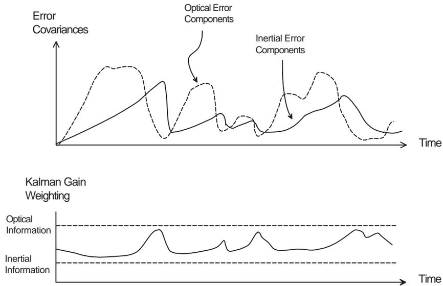
Figure 4.1: Kalman gain matrix dynamically changes weights of input types based on their contributions to the error covariance matrix.
