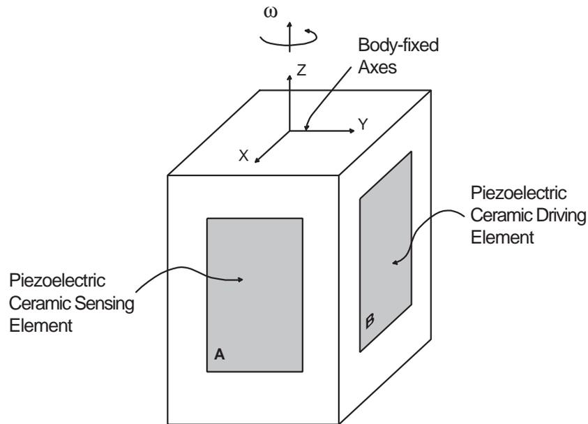
Figure 2.5: A Generalized Vibrating Gyro with Rectangular Cross Section
