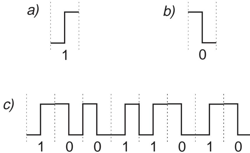
Figure 3.6: Schematized view of PSK: (a) 1-bit, (b) 0-bit, (c) 8 bits: 10011010
