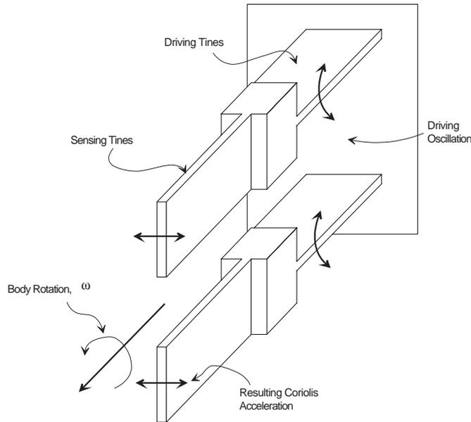
Figure 2.4: Schematic of a tuning fork gyro.
