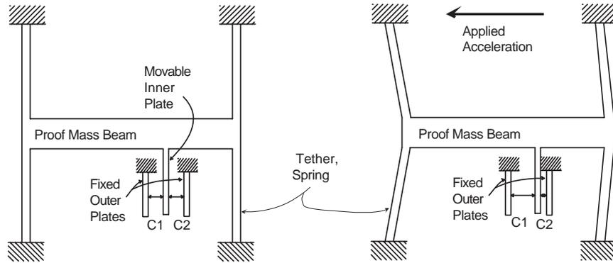
Figure 3.2: Analog Devices' ADXL05 (simplified figure): at rest and under applied acceleration.
