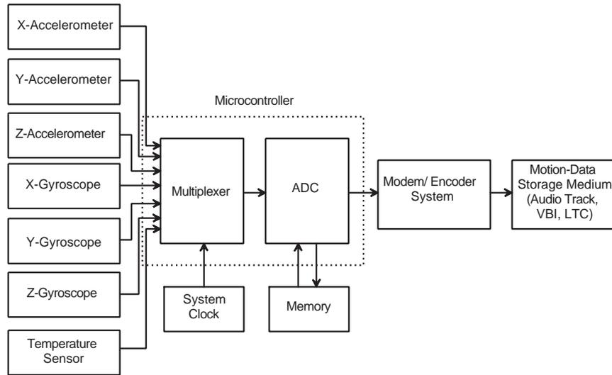
Figure 2.6: Schematic of Inertial Measurement Unit (IMU)
