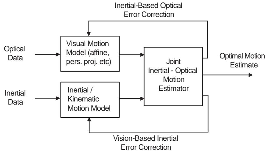
Figure 1.1: Schematic view of the IOME Cam system.
