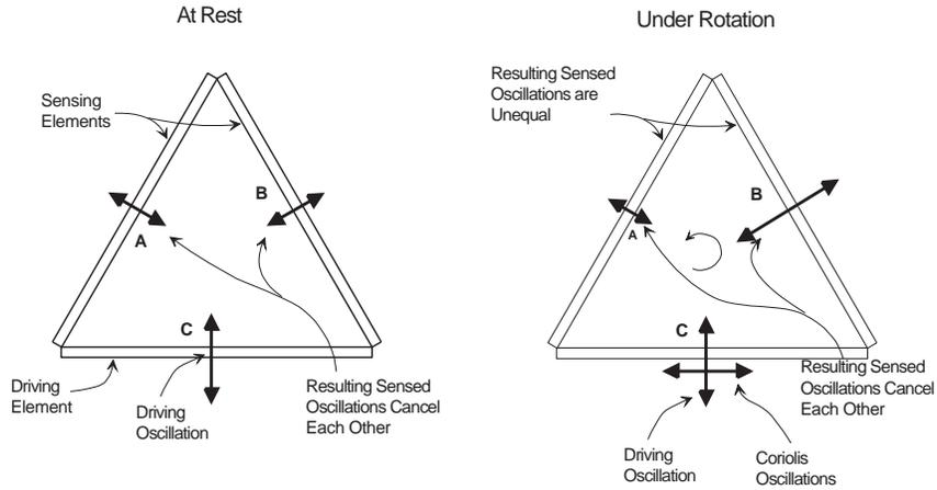
Figure 3.1: An example piezoelectric vibrating gyro: Murata’s Gyrostar.
