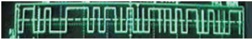
Figure 6-13: Output of continuous-time LFSR circuit
