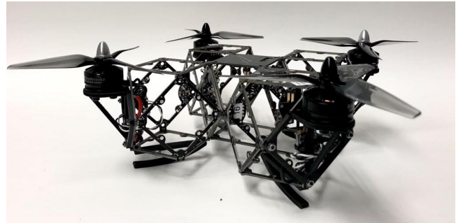
Figure 1: Complete UAS assembled using five voxels
