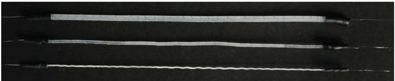
Figure 4: FibeRobo with different diameters of 0.5 mm, 1 mm, and 2.0 mm (bottom to top) plied with conductive wire.
