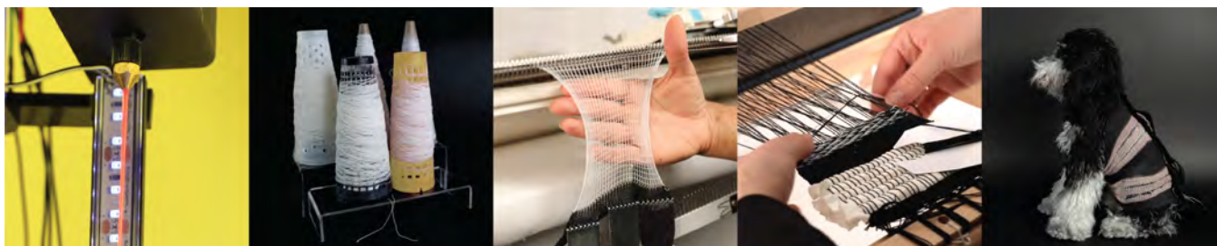
Figure 1: Pipeline from actuating fibers to 4D fabrics. From left to right, 1) FibeRobo being produced in a custom UV drawing machine, 2) 750m of fiber produced in a day, 3) machine knitting with FibeRobo, 4) weaving with FibeRobo, 5) a telepresence canine compression jacket.
