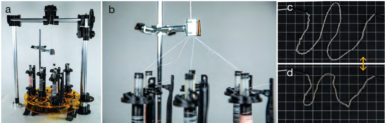
Figure 5: (a) a DIY Maypole braiding machine prepped to produce a braided actuator. (b) a close-up of the braiding process that combines 4 LCE fibers with two litz wires. (c) A 34.5 cm FibeRobo/lite wire braid without electrical power (d) the same braid 8 seconds later, now 21.6 cm, after being powered with 2.5A and 8.5V. Once we remove the power, the fiber returns to its original length after 30 seconds.
