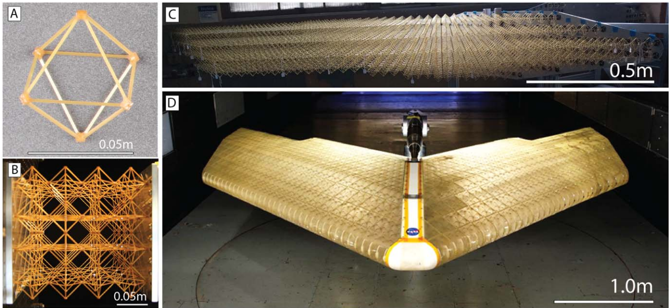
Figure 1. A large-scale, ultralight adaptive structural system. (A) Modular building block unit, (B) 4 \times 4 \times 4 unit cube during mechanical testing, (C) Single half-span wing structure composed of 2088 building block units, (D) Blended wing body aerostructure with skin, mounted to central load balance in the 14 \times 22 subsonic wind tunnel at NASA Langley Research Center.
