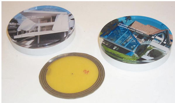
Figure 9 Photograph of the coasters with an exposed resonator in the foreground
